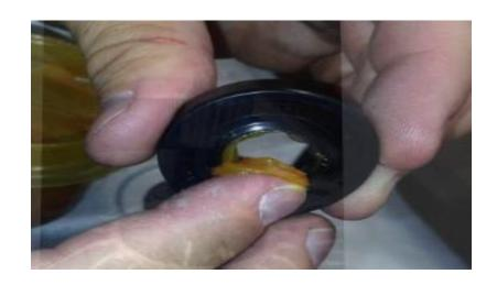
carefully slide the new seal over the input shaft. Press the seal down with your thumbs as evenly as possible.
