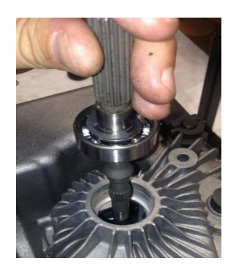
Install the new Input shaft and bearing assembly. Pay attention to the spring that is located inside the unit as this must align correctly.
