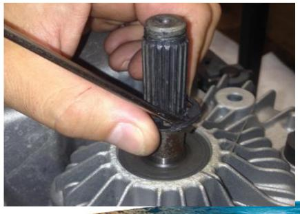
puncturing the seal by puncturing the seal with a screw driver and lifting upward in order to pry out the seal. Be careful not to damage the upper housing.
