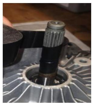
Apply grease to the new oil seal. A generous coating will be fine in order to protect the seal.
