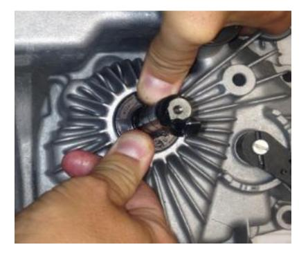
end wrench on the seal and gently tap the seal into proper position.
