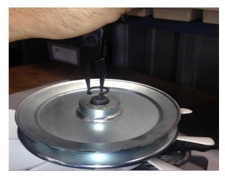
Remove the e-clip from the shaft.
