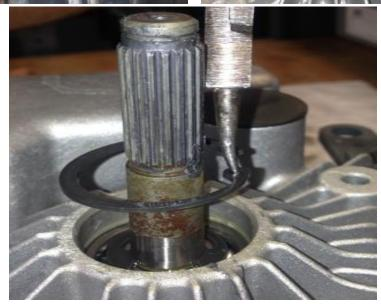
Simply pull the Input shaft and bearing assembly out of the upper housing. Note: Be sure to pull straight out so that you don't move the spring or the pump cylinder block on the inside of the unit. If the internal parts get out of alignment then the unit will have to be completely disassembled.
