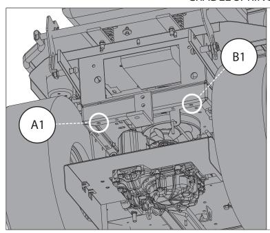
Pre MK4 C Series Tractors may require two cradle springs in order to comfortably lift larger XRD Decks.
