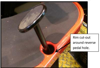
On tractors that don't have this cut-out (prior to serial # A0330761) it is advisable to check if the reverse pedal touches the rim by pressing the forward pedal to its limit. This will cause the reverse pedal to rise up through the running board and if contact is observed then the running board should be changed for one with a cut-out. The part number for the RH running board is:
